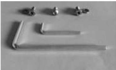
Left side socket head cap with washer, center button cap screw, right side socket head cap with washer, 5mm Allen wrench, 6mm Allen wrench
